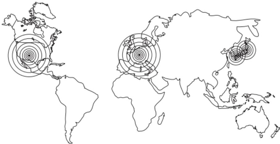
Your Junghans Mega Futura radio-controlled watch is able to automatically receive the radio signals of the following time signal transmitter stations:
