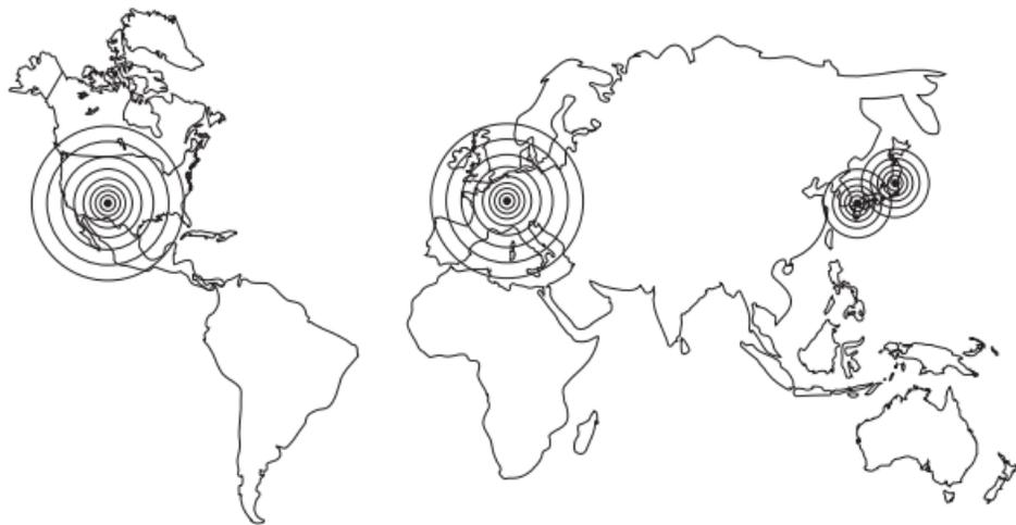
With good reception, the Junghans multi-frequency radio-controlled watch thus always shows the perfectly correct time within any of these four transmission areas. The watch automatically synchronises itself overnight with the DCF77, WWVB, JY40 and JY60 time signal transmitters.
