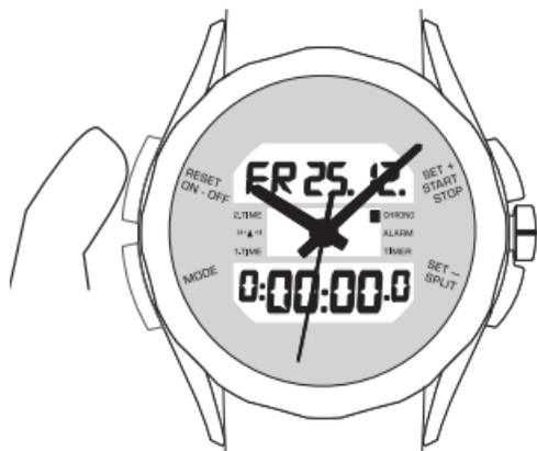
Pressing the 'RESET' button resets the counted time to '0:00:00.0'. The reset function can only be used once the chronograph has already been stopped. When the chronograph is running, the current split time can be displayed by pressing the 'SET-/SPLIT' button for about 5 seconds. The chronograph continues running in the background.
