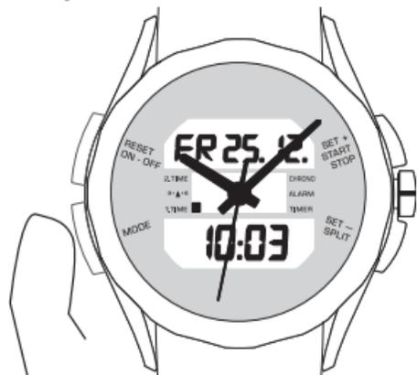
To do so, press the 'MODE' button repeatedly until you reach '1st TIME' mode. The analogue time being shown is now also shown digitally in the bottom part of the LCD display.
