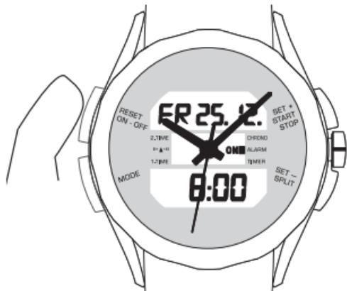
You use the 'ON/OFF' button to turn the alarm on or off. If the alarm is active, the indicator 'ON' is shown in front of the 'ALARM' menu item on the LCD display. When the alarm time is reached an acoustic signal sounds.
