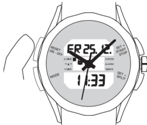
You can protect this function from accidental adjustment by pressing the 'RESET' button for more than 3 seconds. A 'lock symbol' on the LCD display then indicates that the function is 'protected'.
