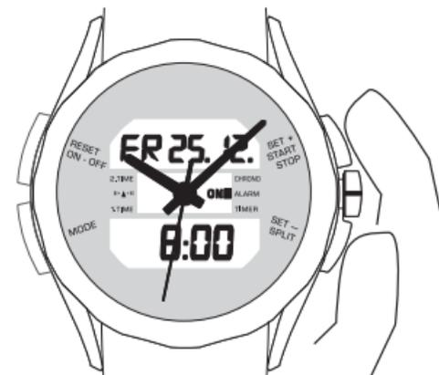
You set the alarm time by using the 'SET+' and 'SET-' buttons. You can adjust the time by the minute by pressing either button briefly or adjust it in fast forward or fast rewind mode by holding the relevant button down for longer.
