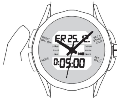
You use the 'ON/OFF' button to turn the timer on or off. If the timer is active, the indicator 'ON' is shown in front of the 'TIMER' menu item on the LCD display. When the timer gets to 0:00:00, an acoustic signal sounds.
