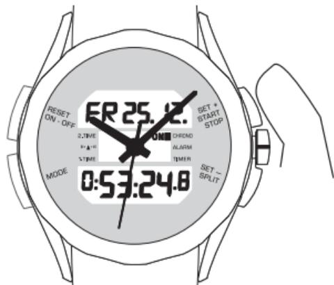
The chronograph is started and stopped again using the 'SET+' button. When the chronograph is running, 'ON' is displayed in front of the 'CHRONO' item on the menu.
